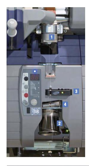
The STS(Spinning Tension Stabilizing)System is a unique and landmark spinning system first used on the VORTEX II 870. Newly developed Friction Roller is equipped in stead of nip roller. More precise control of the drawing of yarn from the spinning. Integrating the clearing zone into the spinning zone results in the optimum spinning monitoring.
